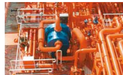
4800 kW LPG Cargo Heater on LPG Vessel, PSHE 9LL-222/1/1 (titanium plates)
