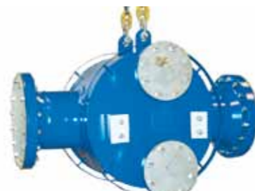
695 kW LNG BOG Heater in a Gas Terminal, PSHE 5LL-124/1/1 (-125 to 200°C Design Temperatures)
