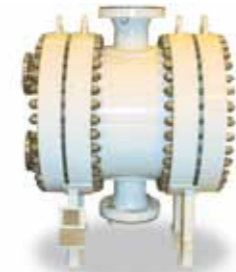
2135 kW 2 nd Stage Suction Cooler (sweet natural gas) operating on a Gas Production Platform, PSHE 7HH-256/1/1 (55 bar design, titanium plates, duplex shell)
