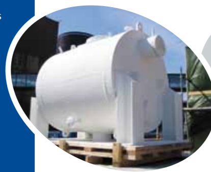
Condensate Preheating PSHE 14HH - 452/2/1 Condensate preheater, 24 MW, before feed water tank
